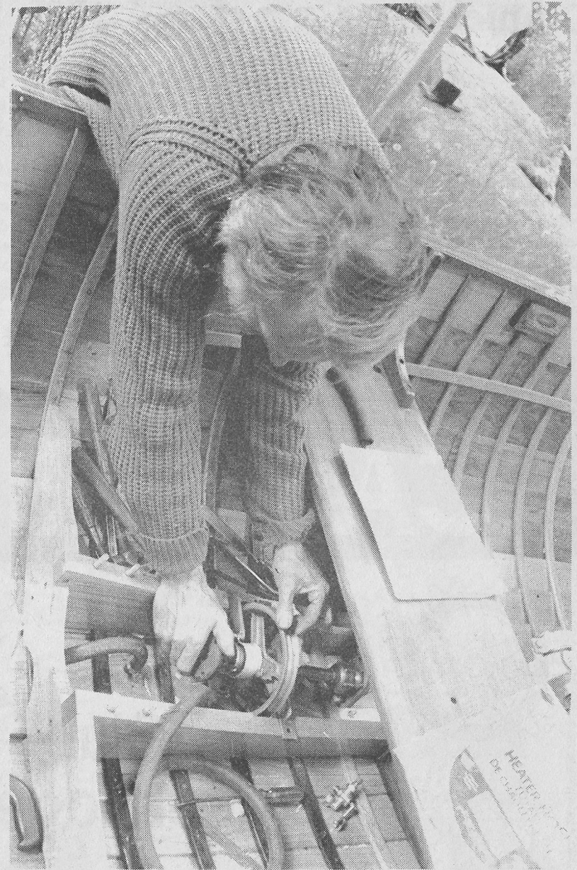
INSTALLING THE HAND CRANK: Paul Dodington has chiselled out spaces in the engine bed to support the hand crank mechanism of a Port Carling dispro. It is important that all the components be secure and accurately lined up to ensure smooth operation and to avoid premature wear. (Tim Du Vernet photo).
